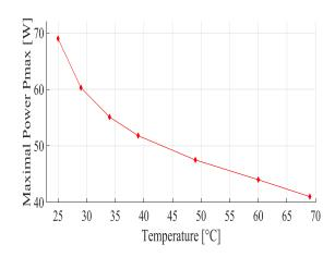
Figure 4. Temperature dependence of maximum power (Pmax)
