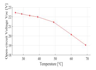
Figure 3. Temperature dependence on open-circuit voltage (Voc)
