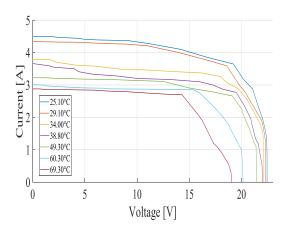
Figure 5. V-I characteristic of a PV panel
