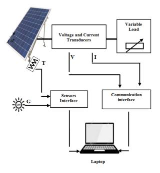
Figure 1. Measurement system setting up
