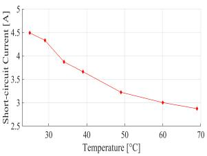
Figure 6. Temperature dependence of Short-circuit current (Isc)
