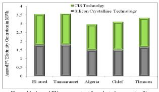
Figure 11. Annual PV energy output for selected areas using Sicrystalline and CIS technology
