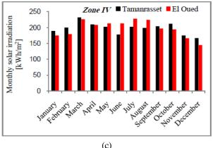
Figure 8. Monthly solar irradiation for each zone at optimal tilt angle, zone I (a), zone II (b), zone IV (c)
