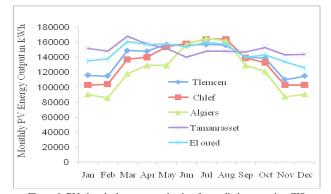
Figure 9. PV electrical energy production for studied areas using CIS technology.
