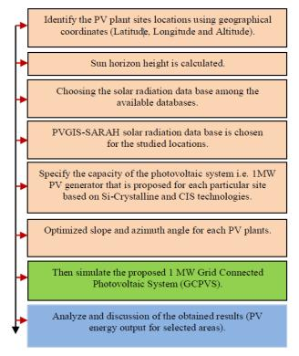
Figure 7. Simulation methodology of 1MW grid connected PV system
