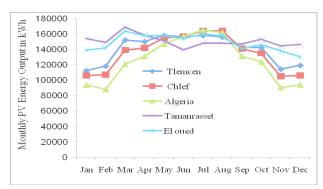
Figure 10. PV electrical energy production for studied areas using Sicrystalline
