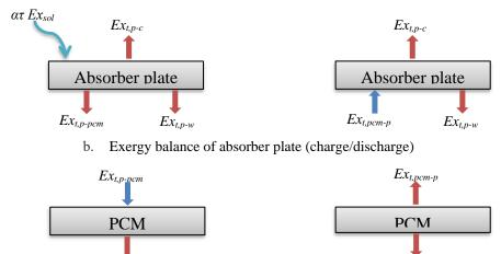
c. Exergy balance of PCM (charge/discharge)
