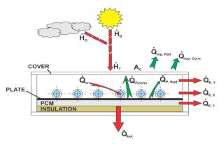
Figure 1. Heat transfer terms involved in solar collector.
