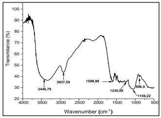
Figure 2, FTIR spectra of coconut fiber biosorbent base activated
