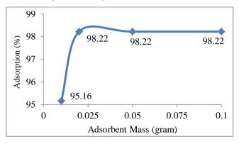
Figure 3. Curve of adsorbent mass variation
