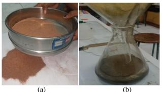
Figure 1. CFB preparation (a) Coconut fiber after mashed, (b) Coconut fiber activated process by immersion with NaOH solution
