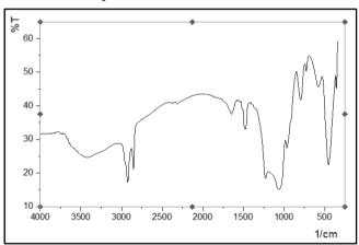
Figure 2. FTIR spectra of synthesized MCM-48
