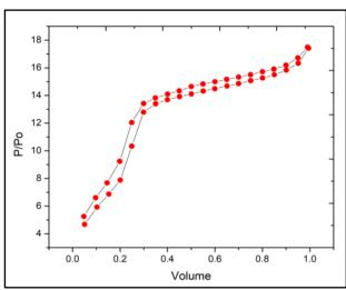
Figure 3. Isothermal N<sub>2</sub> adsorption of MCM-48 before washing
