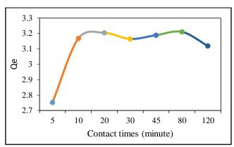
Figure 5. The number of chloramphenicol molecules adsorbed (q<sub>e</sub>) by MCM-48 as a function of contact time
