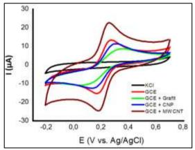
Figure 4. Cyclic voltammogram of 1 mM K<sub>3</sub>FeCN<sub>6</sub> in 0.1 M KCl at glassy carbon and glassy carbon modified with conductive materials by drop coating method.
