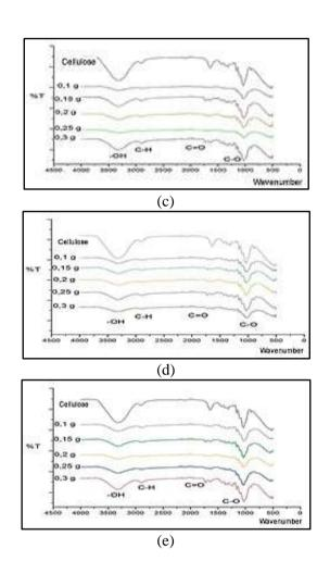
Figure 3. IR spectrum of cellulose, cellulose acetate with variations in the amount of iodine 0.1 - 0.3 grams at time a (1 hour), b (2 hours), c (3 hours), d (4 hours), e (5 hours)
