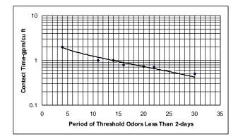
Fig.3: Relationship of Contact Time to Reduction f Threshold Odor at (Nitro, W. Va) (Dostal et al, 1965).
