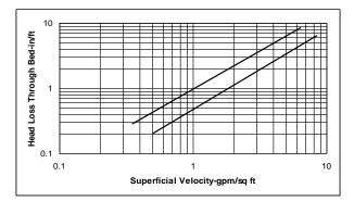
Fig. 5: Head Loss on Coal-Based Granular Bed at 22 °C (Magee, 1956).
