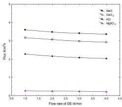
Fig. 7, Effect of flow rate of DS on the flux of water at concentration of DS = 10% by wt , flow rate of FS = 1 lit/min and temperature of FS and  $DS = 20^{\circ}C$
