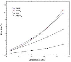
Fig. 2, Effect of DS concentration on the flux of water at temp of FS and DS =  $20^{\circ}$ C, Flowrate of FS and DS = 1 lit/min
