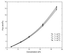
Fig.5 Effect of concentration of  $CaCl_2$  on the flux of water at different temperature of DS, temp of FS = 20°C, flow rate of feed and DS = 1 lit/min
