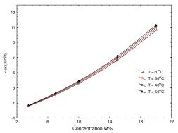
Fig. 4, Effect of concentration of NaCl on the flux of water at different temperature of DS and at temp of feed =  $20^{\circ}$ C, flow rate of feed and DS = 1 lit/min
