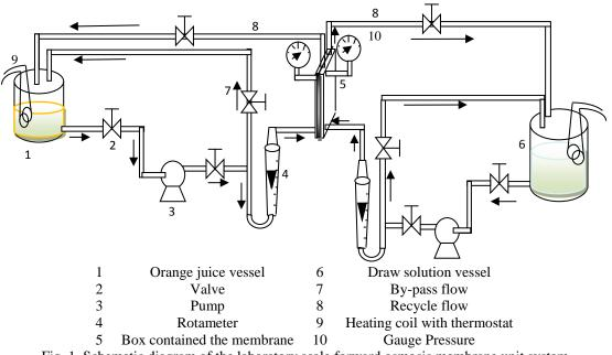
Fig. 1, Schematic diagram of the laboratory scale forward osmosis membrane unit system
