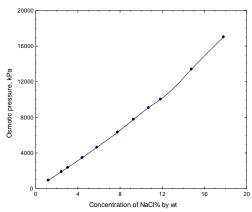
Fig. 9, Osmotic pressure of the Sodium chloride against concentration
