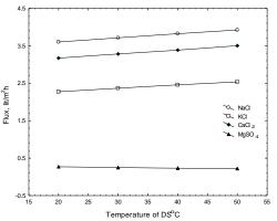
Fig. 3, Effect of Temperature of DS on the flux of water at Concentration of salt in DS = 10%, flow rate of FS and DS = 1 lit/min and at temperature of FS =  $20^{\circ}C$
