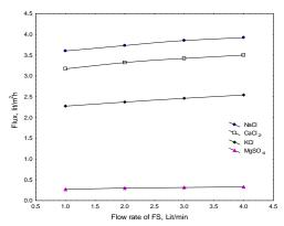
Fig. 6, Effect of flow rate of FS on the flux of water at concentration of DS = 10% by wt, Flow rate of DS = 1 lit/min and temperatures of FS and  $DS = 20^{\circ}C$
