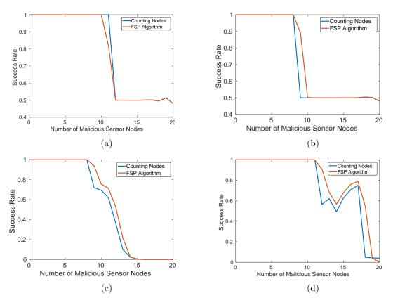
Figure 2: FSP algorithm versus counting sensor nodes technique.
