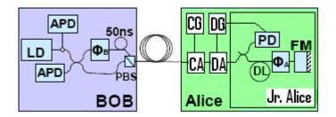
Fig.1: Experimental setup of Weak-Vacuum State Protocol.
