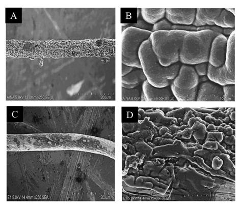
Fig. 4: FESEM images of PEDOT:PSS before (A and B) and after (C and D) chronoamperometry measurement in 0.1 M PBS, pH 7.4, for 10-mm  $\mu$ PtE (after 24 hours).
