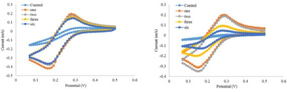
Fig. 1: CV of 10-mm μPtE/PEDOT:PSS in 0.1 M K<sub>3</sub>Fe(CN)<sub>6</sub> solution at a scan rate of 100 mV/s over six days.
