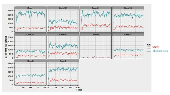
Fig. 4: The Comparison between the Shortest Path and NNTF of the packet drop rate of ten routers, in Kbit.
