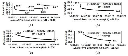
Fig. 3: Loss of Pre-load with Time for Bolt-2. (a) Overall tightening, (b) First tight, (c) First Re-tight, (d) Second Re-tight.
