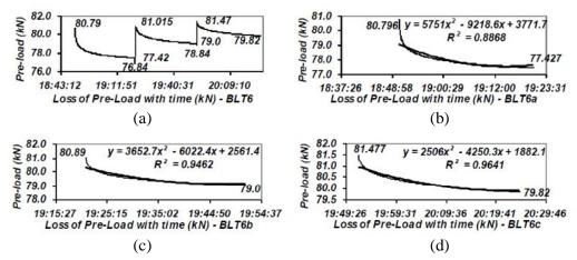
Fig. 5 Loss of Pre-load with Time for Bolt 6. (a) Overall tightening, (b) First tight, (c) First Re-tight, (d) Second Re-tight.
