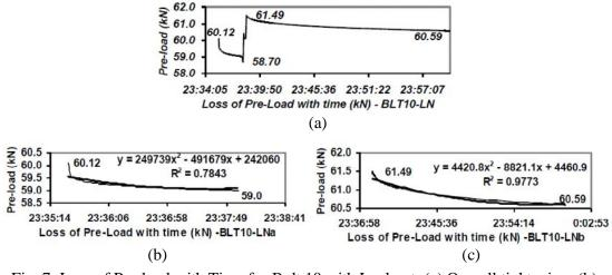
Fig. 7: Loss of Pre-load with Time for Bolt 10 with Locknut. (a) Overall tightening, (b) First tight, (c) First Re-tight.
