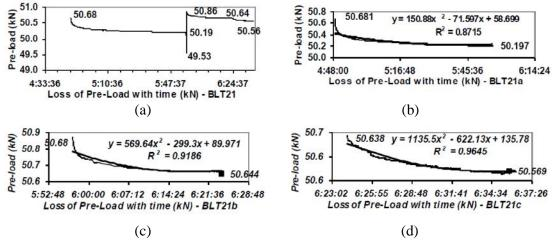
Fig. 8 Loss of Pre-load with Time for Bolt 21. (a) Overall tightening, (b) First tight, (c) First Re-tight, (d) Second Re-tight.
