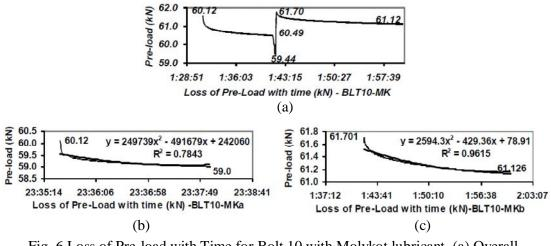
Fig. 6 Loss of Pre-load with Time for Bolt 10 with Molykot lubricant. (a) Overall tightening, (b) First tight, (c) First Re-tight.
