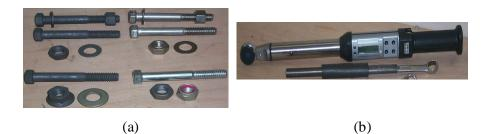
Fig. 2 (a) Bolts, nuts and washers used during tests, (b) Tools (torque wrenches) used.
