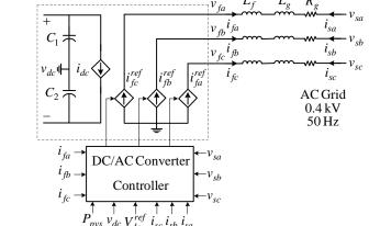
Fig. 5: Average large signal model of the DC-AC converter.
