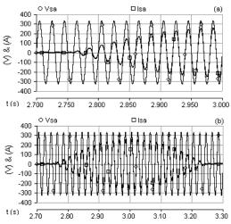
Fig. 10: Grid voltage and injected current for a step change from 1000 to 300 W/m<sup>2</sup> and from 300 to 800 W/m<sup>2</sup>.
