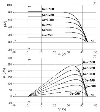
Fig. 3: Characteristic curves of the PV array with different solar irradiations.
