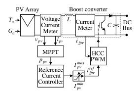
Fig. 4: Proposed control system for each boost converter.
