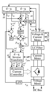
Fig. 6: Control System of the DC-AC converter.
