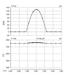
Fig. 14: Frequency variation effect on (a) Output power from the DC bus and (b) DC bus voltage.
