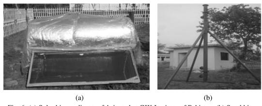
Fig. 6: (a) Solar biogas digester fabricated at GIK Institute of Pakistan, (b) Scrubbing tower for removal of carbon dioxide from biogas.
