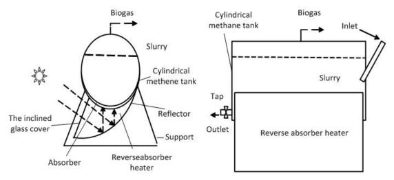
Fig. 5: Schematic diagram of solar biogas digester.
