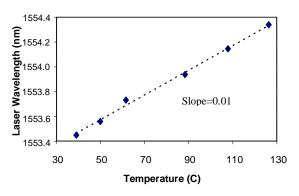
Fig. 4 Fiber laser wavelength against applied temperature
