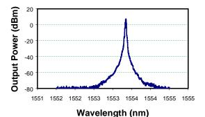
Fig. 3 Spectrum of laser output measured by optical spectrum analyzer
