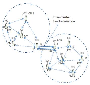
Fig. 9: Proposed Inter-cluster synchronization procedure.
