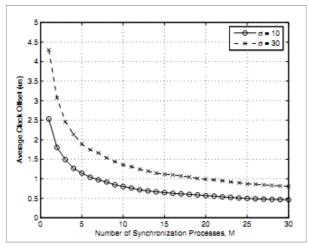
Fig. 5: Average clock offset in different receive delay difference standard deviation,  $\sigma$  [8]
