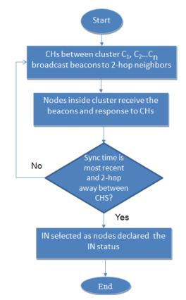
Fig. 8: Proposed Intermediate Node (IN) selection procedure.
