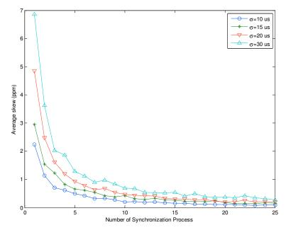
Fig. 12: Average clock skew on different receive delay difference in standard deviation for 50 nodes
