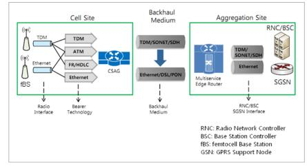
Fig. 2: Femtocell Base Station in wireless backhaul network structure.
