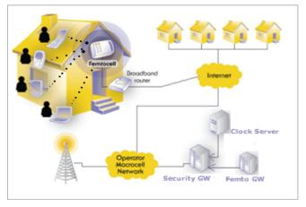
Fig. 1: A femtocell network architecture [2]
