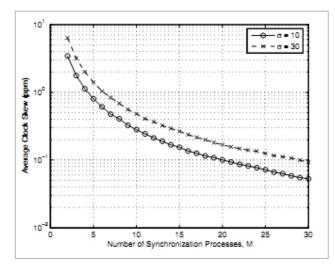
Fig. 6: Average clock skew in different receive delay difference standard deviation,  $\sigma$  [8].
