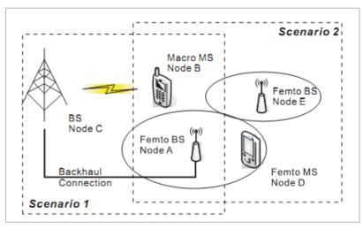
Fig. 4: The Two Femtocell Synchronization Scenarios [8].
