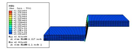
Fig. 4: Contour of shape after blanking process of mild steel 2 mm.
