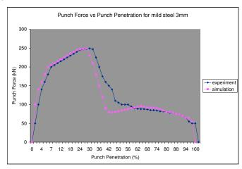
Fig. 7: Simulation compared with experimental results of Hambli and Potiron [12].
