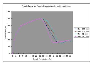
Fig. 9: Simulation of punch force against punch penetration for various punch edge radius for blanking of 3 mm MS sheet.
