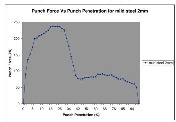
Fig. 5: Punch force vs punch penetration of blanking process (2 mm MS sheet).
