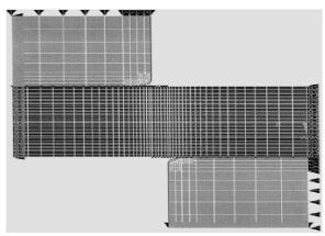
Fig. 2: Mesh in the shearing zone.
