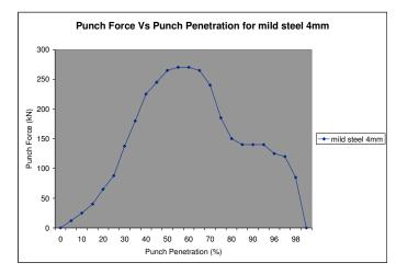
Fig. 6: Punch force vs punch penetration of blanking process (4 mm MS sheet).
