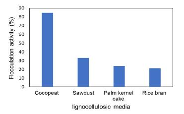
Fig. 4. Flocculation activity of the myco-coagulant in four different lignocellulosic media.
