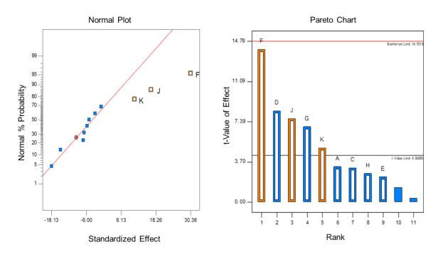
Fig. 6. Pareto chart illustrates the order and significance of the variables affecting flocculation activity using Plackett-Burman design (the blue color represents negative effects, and the orange color represent positive effects).
