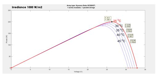
Fig. 12: P-V characteristic curve under variable temperature.
