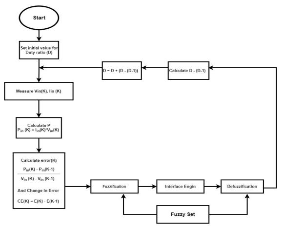
Fig. 6: The operational flow chart of the FLC.
