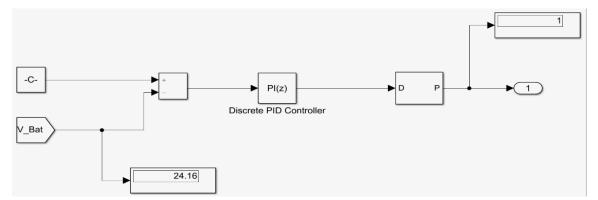
Fig. 8: PI controller for constant voltage supply.
