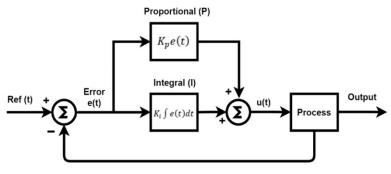
Fig. 2: PI controller block diagram.
