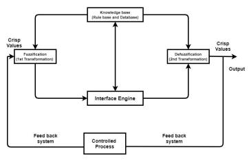
Fig. 1: Block diagram for FLC.
