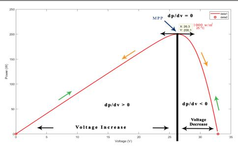
Fig. 5: Power vs voltage characteristic for MPPT algorithm.
