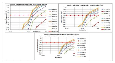
Fig. 3: Power Received (dBm) vs Availability for different elevation angles at certain values of beam divergence angle.
