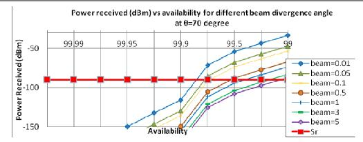
Fig. 4: Power Received vs Availability for different beam divergence angle at  $\theta$ =70°.
