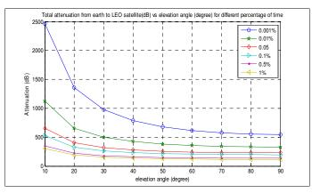
Fig. 1: Total Attenuation vs elevation angle for different percentage of time.
