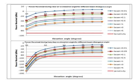
Fig. 2: Power Received (dBm) vs elevation angle (degree) for different beam divergence angle during clear air and during hazy days.
