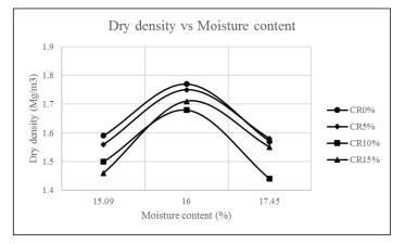
Fig. 6: Compaction curve.
