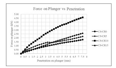
Fig. 7: California Bearing Ratio result.
