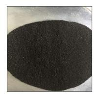
Fig. 2: 40 mesh of crumb tyre rubber.
