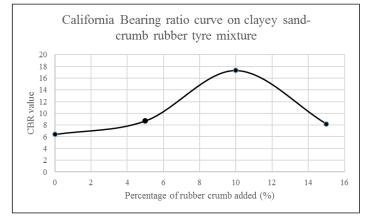
Fig. 8: Effect of percentage of crumb rubber added on CBR value.
