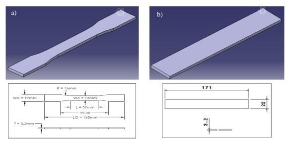
Fig. 1: (a) Part A (above: geometry, below: dimension) and (b) Part B (above: geometry, below: dimension).
