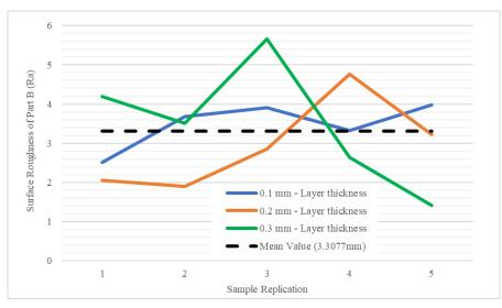
Fig. 4: Trend of surface roughness measurement for Part B.
