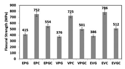
Fig. 4: Flexural strength analysis of E-glass / carbon fiber reinforced IPN (EP/VP/EV) laminate.
