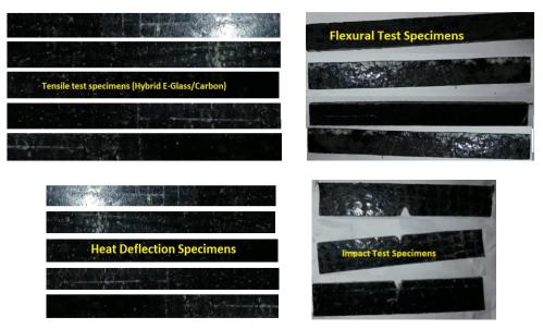
Fig. 2: Hybrid test specimens of IPN composite.
