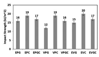
Fig. 5: Impact strength analysis of E-glass/carbon fiber reinforced IPN (EP/VP/EV) laminate.
