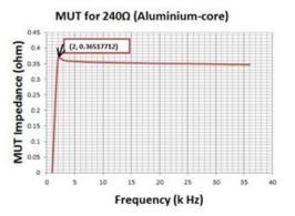
Fig. 17: Resistive materials under test with a load resistance of 240  $\Omega$  for aluminium-core.
