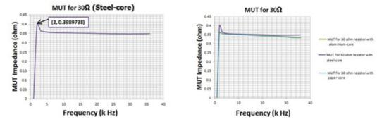
Fig. 14: Resistive materials under test with a load resistance of  $30 \Omega$  for steel-core.
