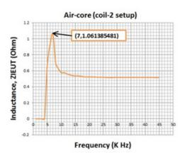
Fig. 8: Inductive peak against frequency variation for aircore coil-2 setup.
