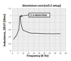
Fig. 9: Inductive peak against frequency variation for aluminium-core coil-2 setup.
