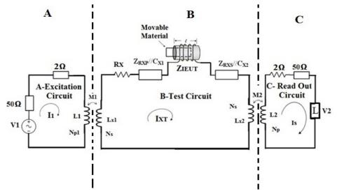
Fig. 2: Schematic representation of the circuit diagram.
