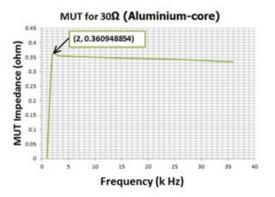
Fig. 13: Resistive materials under test with a load resistance of  $30 \Omega$  for aluminium-core.
