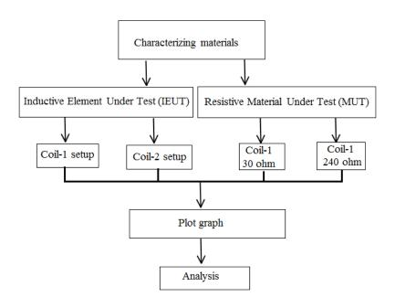
Fig. 3: Flowchart of the experimental setup.
