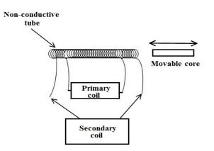
Fig. 1: Material testing coil.
