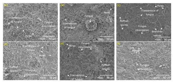
Fig. 3: SEM micrographs at 500× magnification of cross-linked mango seed starch films with various citric acid concentrations (a) 0, (b) 2, (c) 4, (d) 6, (e) 8, and (f) 10 wt.%.
