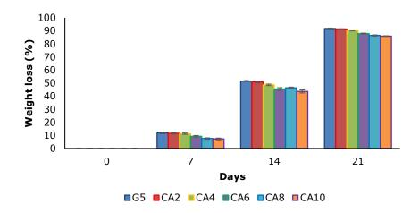
Fig. 4: Weight loss of non-cross-linked and cross-linked mango seed starch-glycerol films after buried in soil for 21 days.
