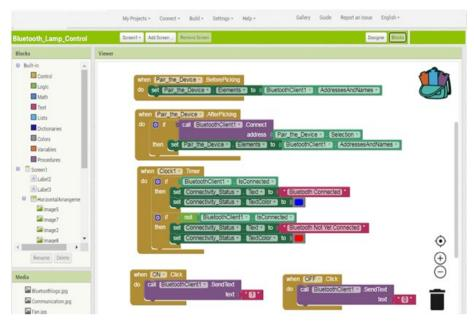
Fig. 3: Android application developed.
