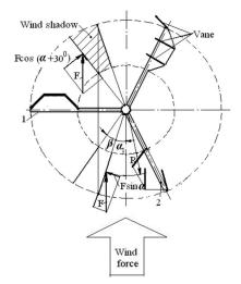
Fig. 3: Vane type wind turbine of three frames.
