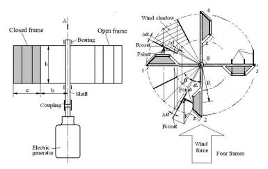
Fig. 2: Vane type wind turbine of four frames.
