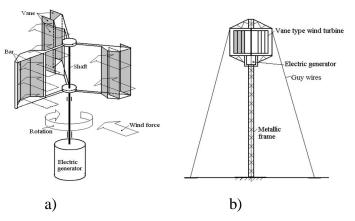
Fig. 1: a) Sketch of the vane type wind turbine, b) and general view of wind station.
