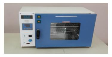
Fig. 5:.Curing and drying furnace.
