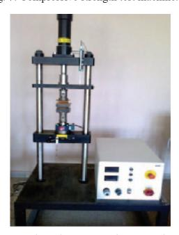
Fig. 8: Sample under compressive strength test.
