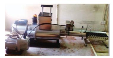
Fig. 4: Clay extrusion device.
