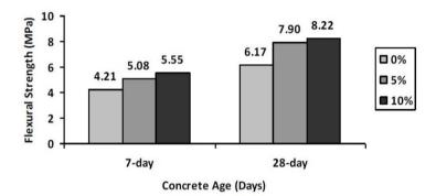
Fig. 3: Flexural strength result of POC concrete and conventional concrete [9].
