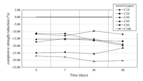
Fig. 1: Concrete strength performance with POC as replacement of coarse aggregates [8].
