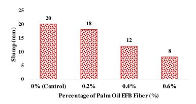
Fig. 8: The slump value with various percentage of reinforced palm oil EFB fiber.
