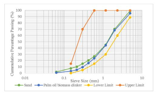
Fig. 7: Particle size distribution of sand and POBC.
