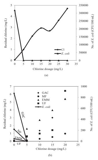
Fig. 4: Chlorination curve profile for (a) raw effluent and (b) pre-treated raw effluent.
