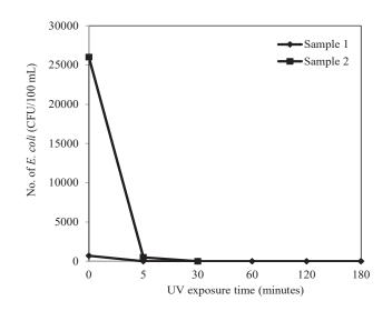
Fig. 3: Effect of UV exposure time towards *E. coli* removal for different raw effluent quality.
