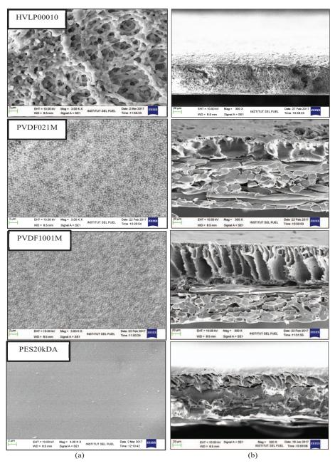
Fig. 6: (a) Surface morphology and (b) cross-sectional micrographs of flat sheet commercial membranes at the magnification of 3000x and 300x, respectively.
