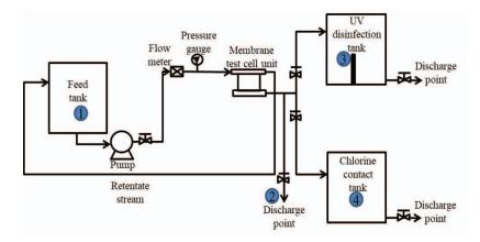
Fig. 1: Schematic diagram of bench-scale integrated disinfection system (MF/UFchlorination and MF/UF- UV) with sampling points: (1) at feed tank (2) at discharge point after the membrane unit (3) at UV disinfection tank (4) at chlorine contact basin.
