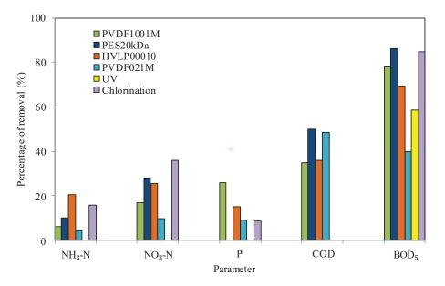
Fig. 5: Performance of single disinfection unit.
