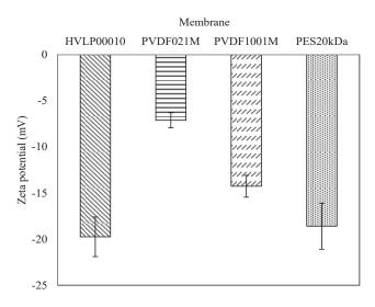
Fig. 7: Membrane surface charge for the commercial flat sheet membranes.
