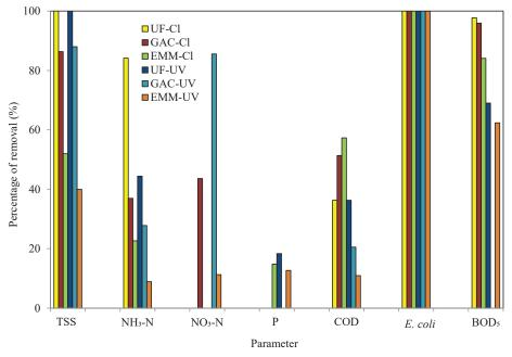
Fig. 8: Performance of integrated disinfection system.
