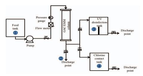
Fig. 2: Schematic diagram of bench-scale integrated disinfection system (GAC/EMM column-chlorination and GAC/EMM column–UV) with sampling points: (1) at feed tank (2) at discharge point of GAC/EMM column (3) at UV disinfection tank (4) at chlorine contact basin.
