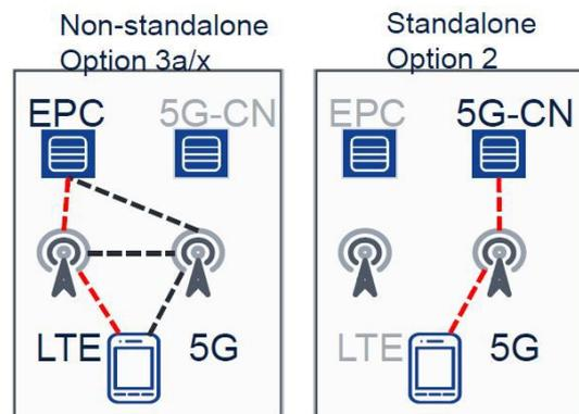
Fig. 5: Proposed 5G architectures in 3GPP Release 15 [31].
