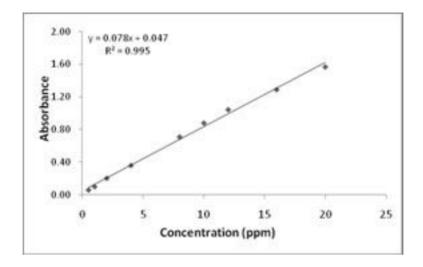
Fig. (6): Calibration graph of paracetamol.
