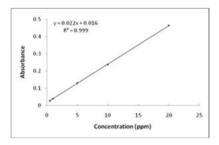
Fig. (3): Calibration graph of paracetamol
