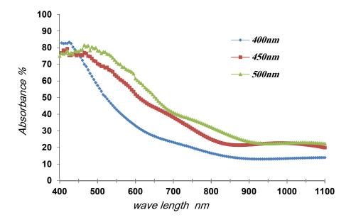
Figure. (3): Absorption spectra of ZnTe thin films with different thicknesses
