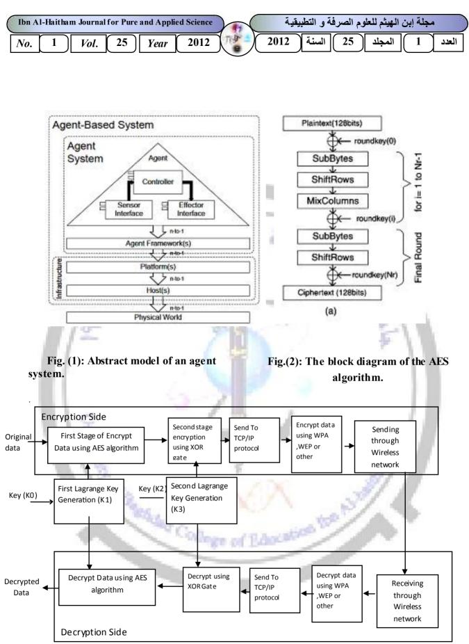
Fig.(3): The proposed Agent Connection Encryption/Decryption System
