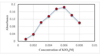
Figure (3): The effect of potassium periodate concentration on the color development in the determination of 20 µg.mL<sup>-1</sup>(CRN.).
