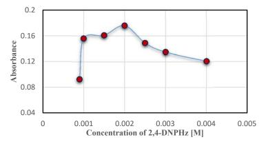
Figure (2): The effect of the concentration of 2,4-DNPHz on the color development in the determination of 20 µg.mL<sup>-1</sup> (CRN.).
