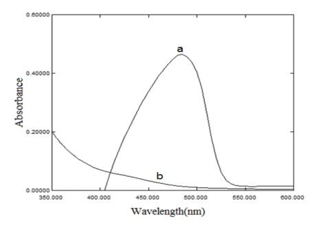
Figure (6): Absorption spectra of: (a) 20 μg.mL<sup>-1</sup>(CRN.) against reagent blank, (b) blank solution against solvent under the optimum conditions.
