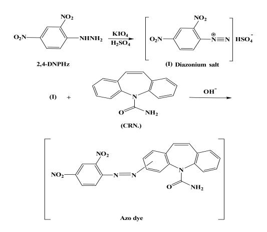
Scheme (2): The suggested reaction mechanism between (CRN.) and 2,4-DNPHz.
