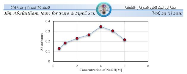
Figure (4): The effect of sodium hydroxide concentration on the color development in the determination of 20 µg.mL<sup>-1</sup>(CRN.).
