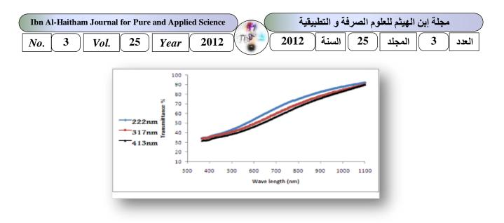
Fig.(3): Transmission as function of wavelength for ZnO films with different thicknesses
