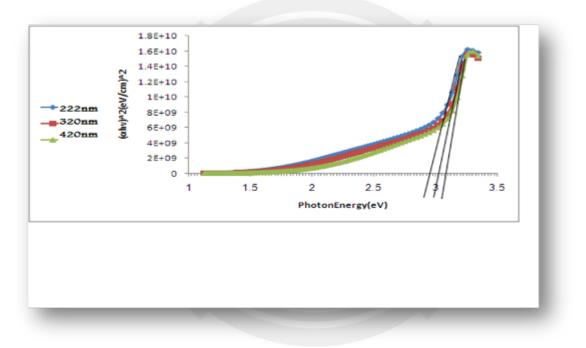
Fig. (4): A plot of  $(\alpha hv)^2$  as function of photon energy for ZnO films with different thicknesses
