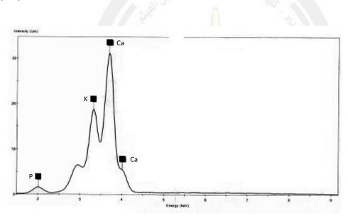
Fig. (4): XRF analysis of wet HA sample prepared with molar ratio (1:1)
