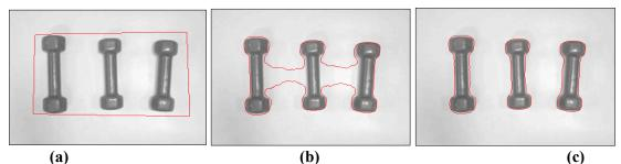
Fig. (2): Segmenting three weights far from each other, (a) input image with the initial front, (b) initial front evolution, (c) segmentation results.
