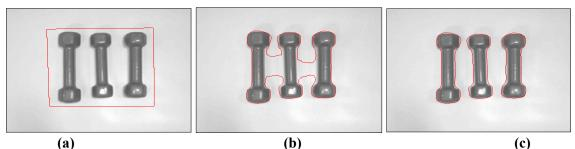
Fig. (3): Segmenting three weights close to each other, (a) input image with the initial front, (b) initial front evolution, (c) segmentation results.
