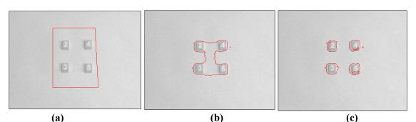
Fig. (15): Segmentation process of four square objects with a color similar to the background color to a large extent with medium illumination, (a) input image with the initial front, (b) initial front evolution, (c) segmentation result
