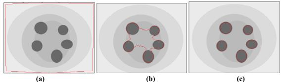
Fig. (12): Segmenting five circular objects located inside three combined circles with significant colorific difference, (a) input image with the initial front, (b) initial front evolution, (c) segmentation result.
