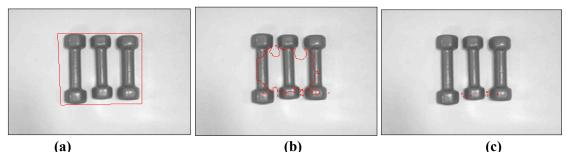
Fig. (6): Segmenting three weights very close to each other, (a) input image with the initial front, (b) initial front shrank after 120 iterations, (c) initial front vanished after 250 iterations
