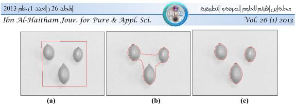
Fig. (17): Segmentation process of three lemons with high illumination, (a) input image with the initial front, (b) initial front evolution, (c) segmentation result
