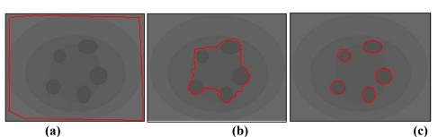
Fig. (9): Segmenting five circular objects located inside three combined circles with simple colorific difference, (a) input image with the initial front, (b) initial front evolution, (c) segmentation result.
