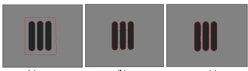
(a) (b) (c) Fig. (8): Segmenting three objects very close to each other, (a) input image with the initial front, (b) initial front evolution, (c) segmentation result
