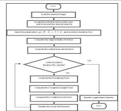
Fig. (1): Overview diagram of the modified geometric deformable model
