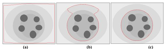
Fig. (11): Fail segmentation process of five circular objects located inside three combined circles with significant colorific difference, (a) input image with the initial front, (b) initial front evolution after 380 iterations, (c) wrong final segmentation result after 600 iterations.
