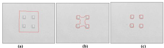
Fig. (14): Segmentation process of four square objects with a color similar to the background color to a large extent with high illumination, (a) input image with the initial front, (b) initial front evolution, (c) segmentation result
