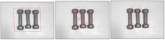
(a) (b) (c) Fig. (7): Segmenting three weights very close to each other, (a) input image with the initial front, (b) initial front evolution, (c) segmentation result.
