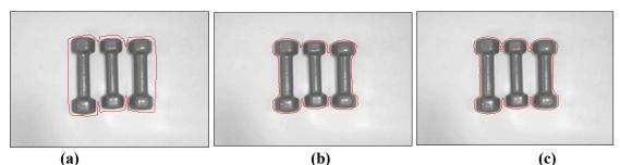
Fig. (5): Segmenting three weights very close to each other, (a) input image with the initial front permeates the distance between objects, (b) initial front evolution, (c) wrong segmentation results
