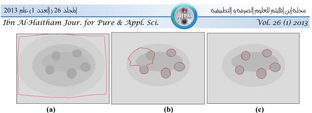
Fig. (10): Segmenting five circular objects located inside three combined ellipses with simple colorific difference, (a) input image with the initial front, (b) initial front evolution, (c) segmentation result.
