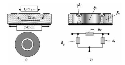
Figure (1): (a) Shape of the specimen and of the electrodes.
