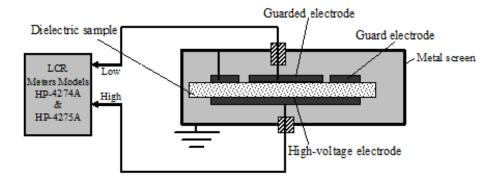
Figure (3): Schematic diagram for the A.C. measurements.
