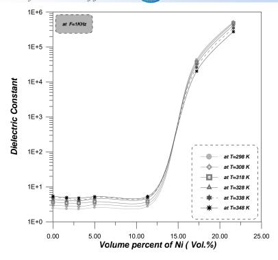
Figure (10): Variation of dielectric constant,  $\varepsilon'$ , of *PE-Ni* composites with the filler concentration & temperature at F=1KHz.
