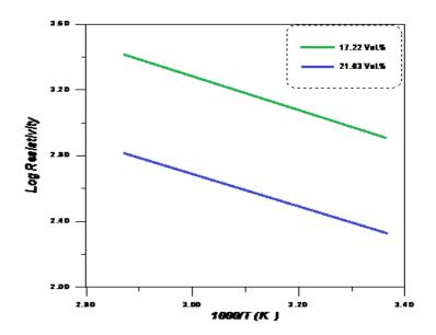
Figure (8): Variation of the volume electrical resistivity,  $\rho_{v}$ , with reciprocal temperature for *PE* specimens of high nickel concentration (i.e. 17.22 & 21.63 Vol.%).
