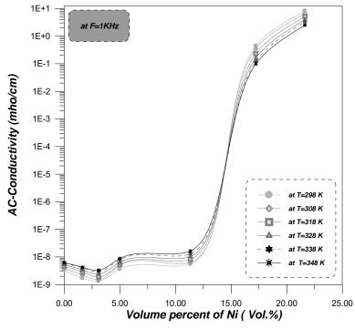
Figure (11): Variation of the A.C conductivity,  $\sigma_{AC}$ , of *PE-Ni* composites with the filler concentration & temperature at F=1 kHz.
