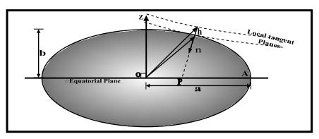
Figure No.(1) Ellipsoidal model of earth (cross-section normal to equatorial plane) [13]
