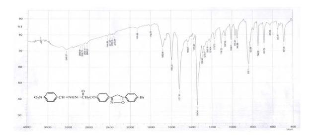
Figure No. (3): FTIR-Spectrum of compound  $[V]_b$
