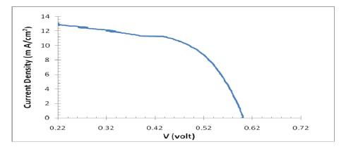
Figure No. (4): Current density-Voltage curves of the (n-CdO:In/p-Si) solar cell
