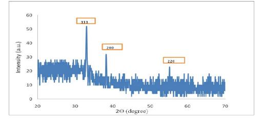
Figure No. (1): XRD of CdO:In thin film on glass substrate
