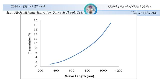
Figure No. (2): The optical transmission (T%) as a function of wavelength for CdO:In film
