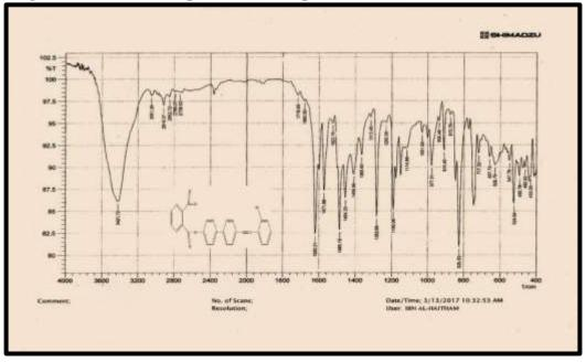
Figure (2): The FT-IR spectrum of the phenolic Schiff base.
