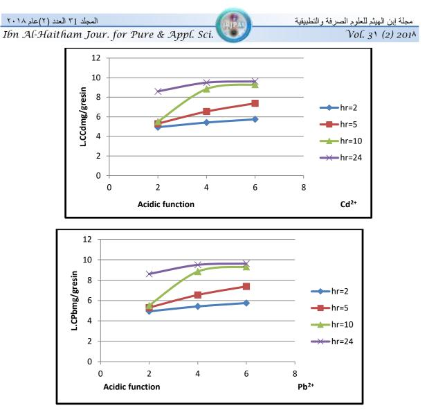
Figure (11): Effect of pH on the load capability of chelate polymer(trinity) on metal ions  $(Ni^{2+}, Cd^{2+}, Pb^{2+}, Cr^{3+})$  in different intervention times
