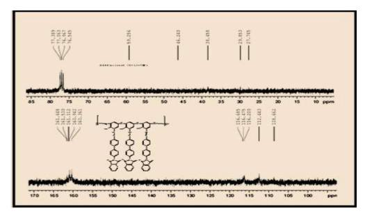
Figure (8): The <sup>13</sup>C NMR spectrum of the phenolic Schiff base resin
