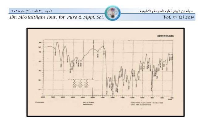
Figure (3): The FT-IR spectrum of the phenolic Schiff base resin.
