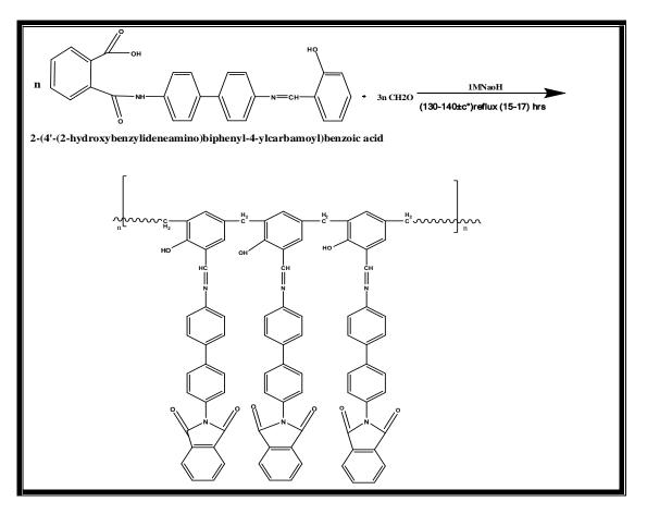
Scheme (3): Structure of the phenolic–Schiff base formaldehyderesins.
