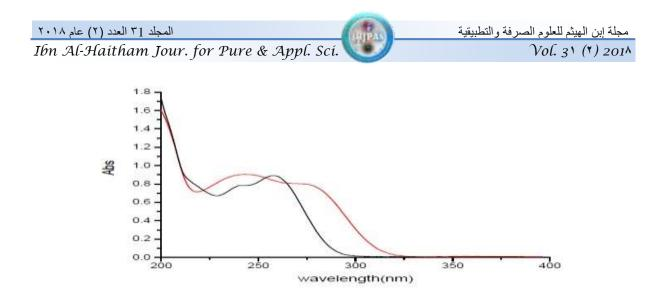
Figure (2): zero order spectra of 4-Aminoantipyrine 30 mg/l(red) and acidic product 30 mg/l (black).
