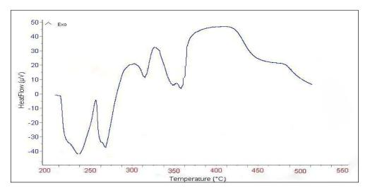
Figure No.(9): DSC curve of polymer (Pi-a2)
