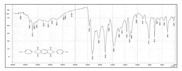
Figure No.( 2 ): FTIR spectrum of (M2).
