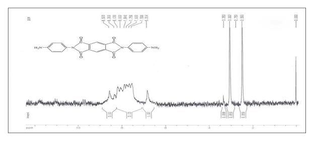
Figure No. (3): <sup>1</sup>H-NMR spectrum of (M2)
