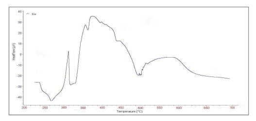
Figure No.(10) : DSC curve of polymer (Pi-a3)
