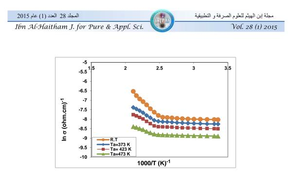
Figure No. (3): lnσ versus 10<sup>3</sup>/T as a function of annealing temperature for (CdTe) films
