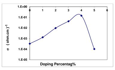
Figure No.( (2): Electrical conductivity as a function of doping ratio for (CdTe) films
