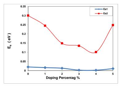
Figure No.(4): Variation activation energies as a function of doping ratio for (CdTe) films
