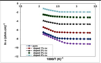
Figure No.(1): Variation lnσ versus 10<sup>3</sup>/T as a function of doping ratio for (CdTe) films
