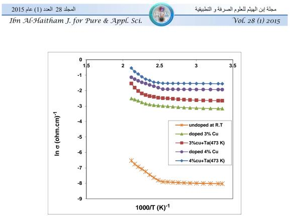
Figure No. (7): lnσ versus 10<sup>3</sup>/T for (CdTe) films un-doped and Cu-doped before and after annealing.
