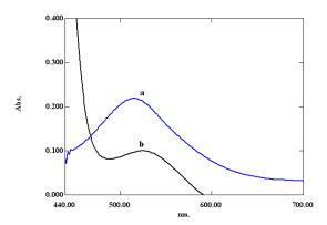
Fig. (2): Absorption spectrum of color product: (a) 15μg.mL<sup>-1</sup> Doxycycline against reagent blank, (b) blank solution against distilled water under the optimum conditions.
