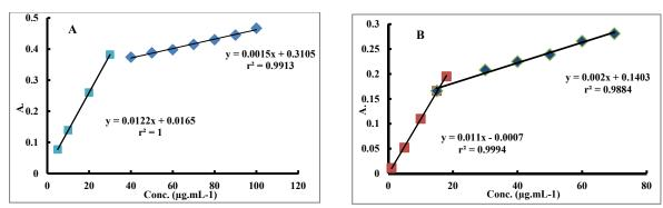
Fig. (4) Calibration curve for the determination of Tetracycline (A) by DOE optimal condition, (B) by univariate optimal condition.
