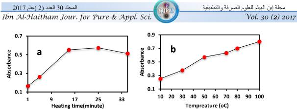
Figure (4): (a) Effect of heating time. (b)Effect of temperature on the absorbance of  $10\mu g.mL^{-1}$  of CLNZ.
