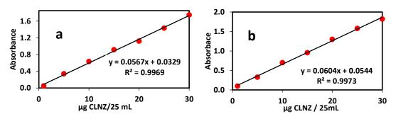
Figure (6): Calibration graph for CLNZ by (a) univariate method (b) the simplex condition.
